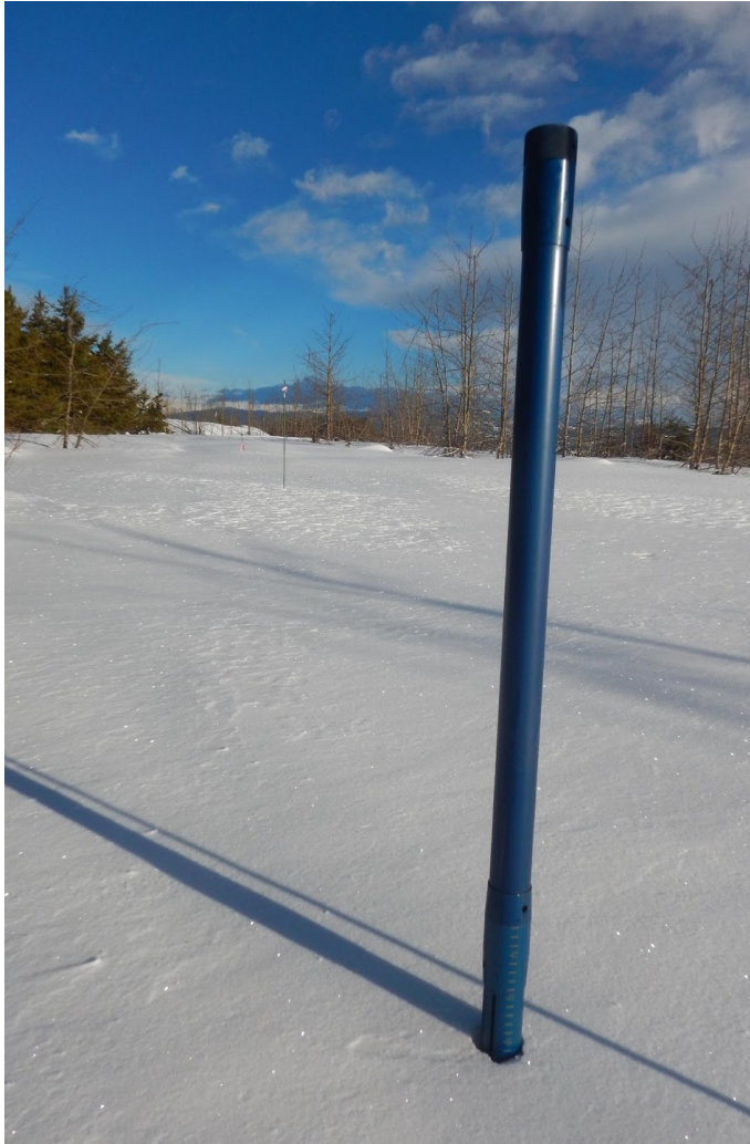
Figure 1 Snow corer for evaluating snowpack.
